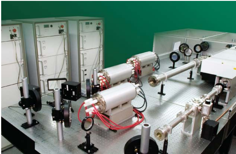
160 J @ 1053 nm MM laser system
